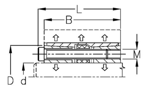
$\begin{array}{lll} \text{B mm} & = 102 \\ \text{d H8 mm} & = 80 \\ \text{D mm} & = 120 \\ \text{Fit tolerance} & = \text{Aksel h8, Nav H8} \\ \text{F kN torque} & = 400 \\ \text{L mm} & = 112 \\ \text{M mm} & = \text{M10} \\ \text{P N/mm2 surface pressure on shaft/hub} = 85 \end{array}$
